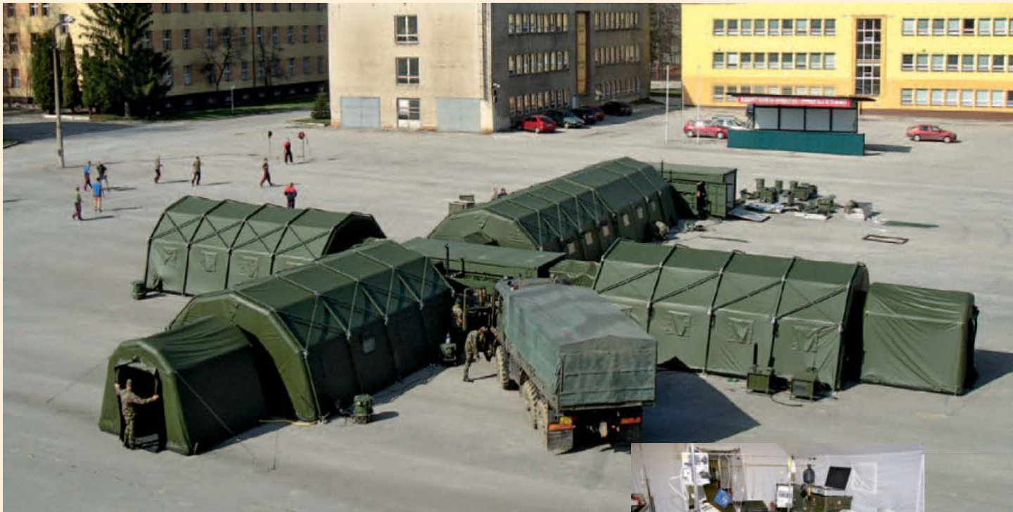
Rapid Deployment System with power supply, air conditioning, CBRN-protection and a total working area of more than 200 m 2 , stored in one container.
