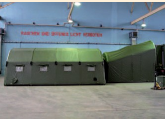
Sluice connection Tent – Container which is operated on a vehicle
