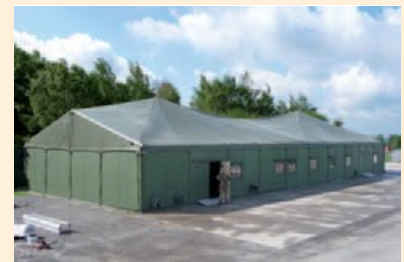
Service Tent, 300 person-design, with rigid outside walls and sun roof
