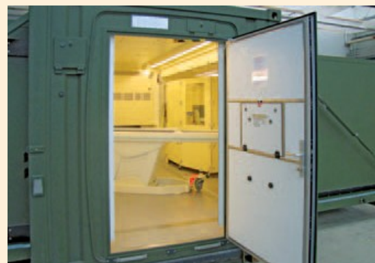
Expandable container type 1:3, for mobile CT-application
