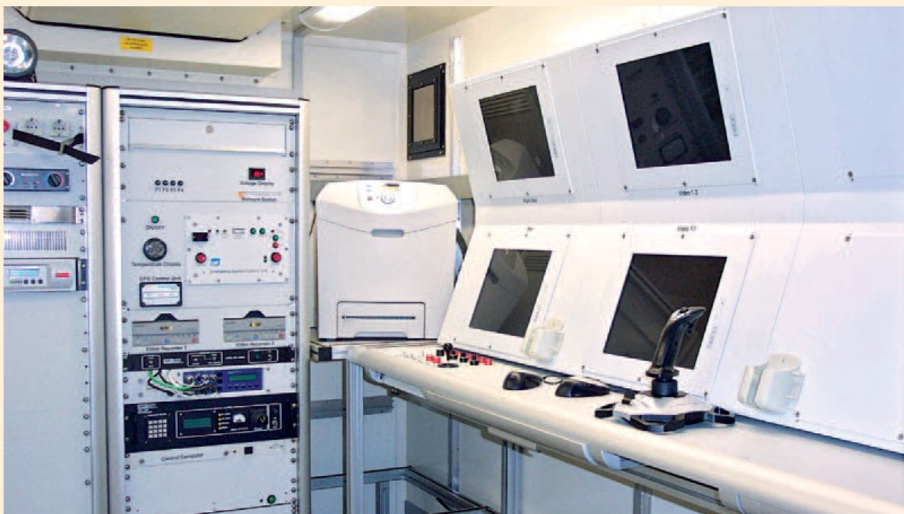
Interior fitting as mobile ground control station for UAV (Drohne)
