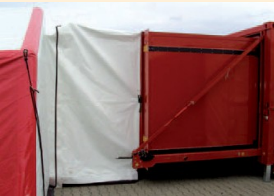
Operation command centre with connected Air Supported Tent type LGZ light
