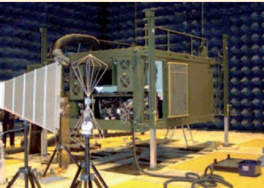
System measurement in absorber hall
