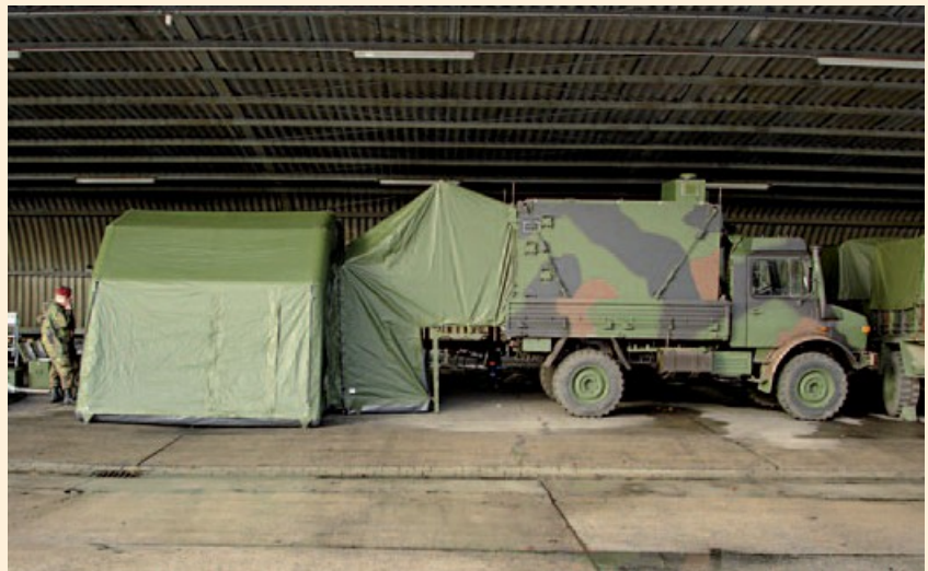
CBRN protected sluce system: vehicle body to Air Supported Tent Type LGZ
