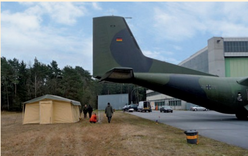
Wind load test by the German Forces at a frame supported Tent type KF22
