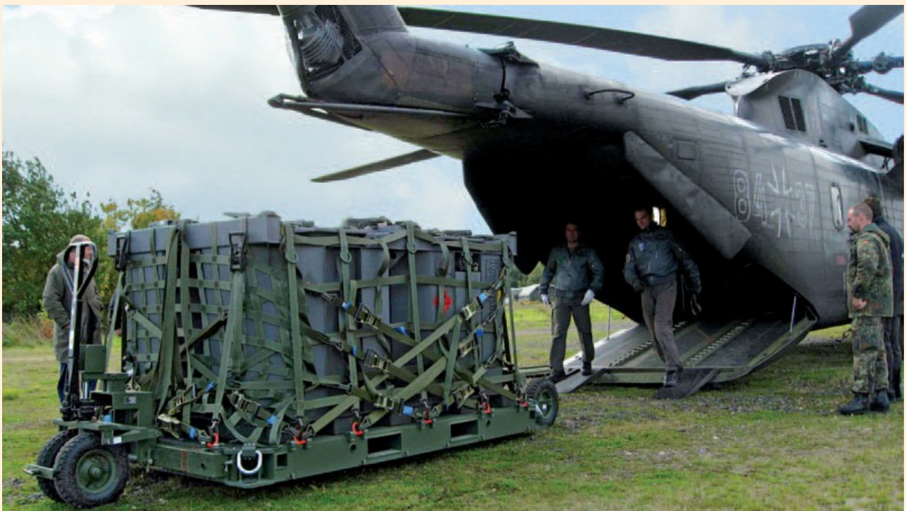
UTP (with installed ground wheel system) during loading procedure into CH53 aircraft
