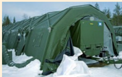
UTP with rigid installation while moving into Air Supported Tent type LGZ
