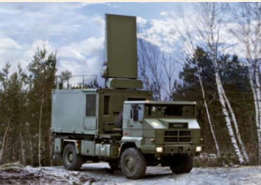
Shelter for mobile radar systems
